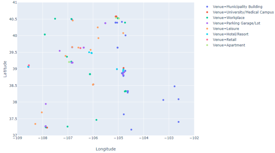
Figure 22: This map is an accompaniment to the previous Figure. It shows the position of every charging station's location, as well as the venue type for each location. This shows that both the number of stations and venue type are important for determining energy usage.
