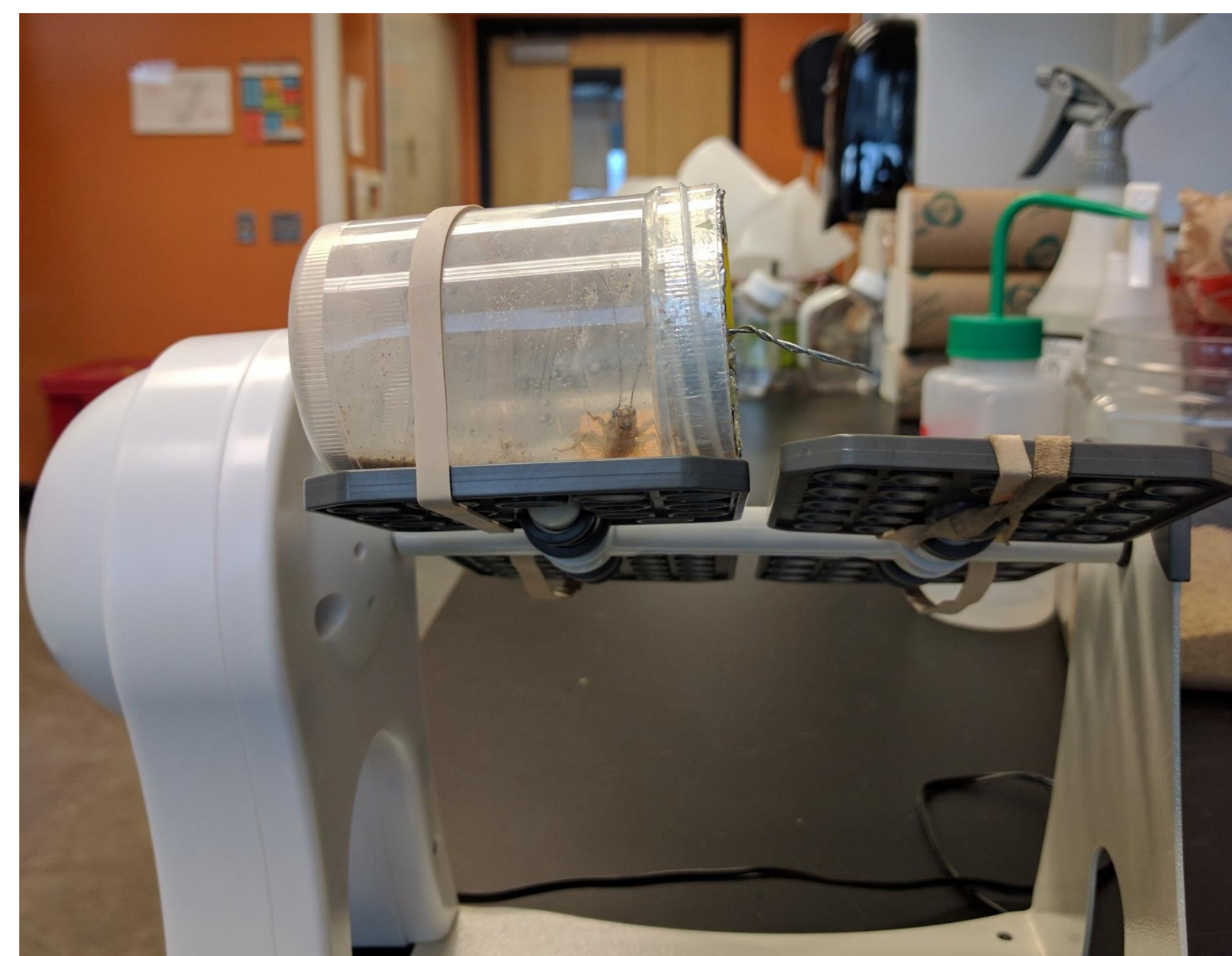
120 mL container attached to rotating rack and rotated.
